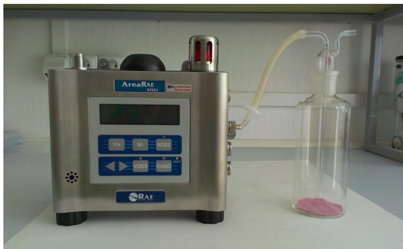
Figure 1. Laboratory arrangement for the amyl acetate desorption from textile materials
