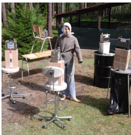
Figure 2. Arrangement of the testing area for the measurements of amyl acetate desorbing from clothes in an open environment
