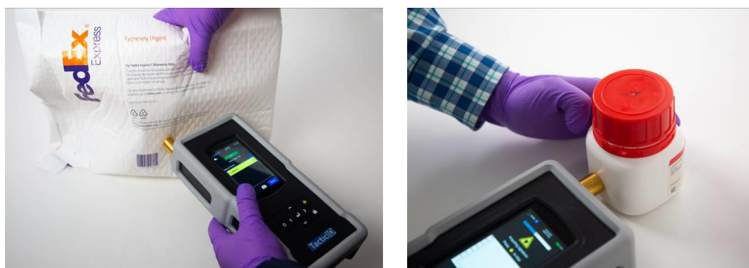
Figure 3 – Raman spectrometer TacticID1064 ST with the accessory for measurements through non transparent packaging
