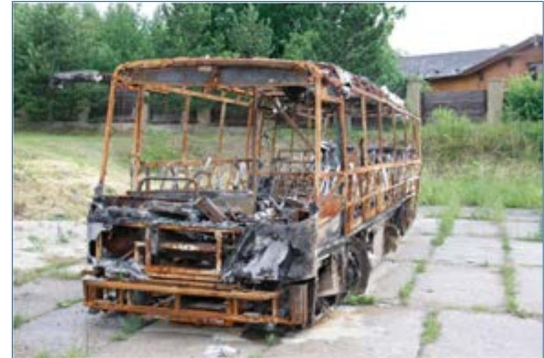
Figure 2 – CNG bus after the fire.
