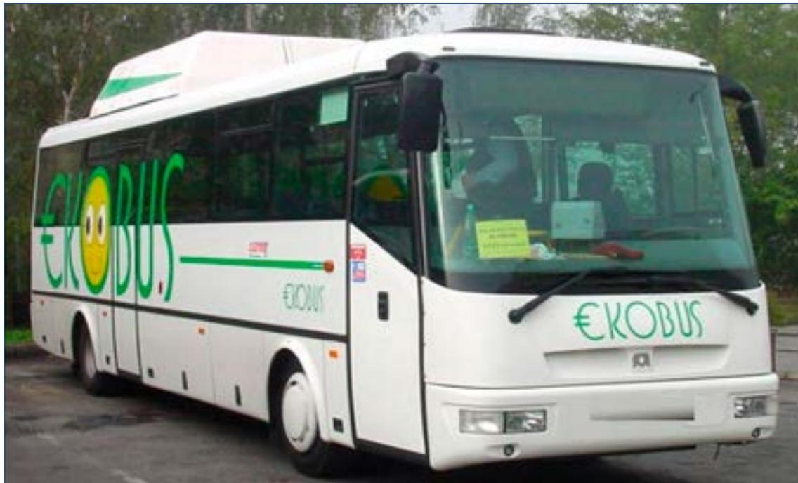
Figure 1 – the CNG bus.
