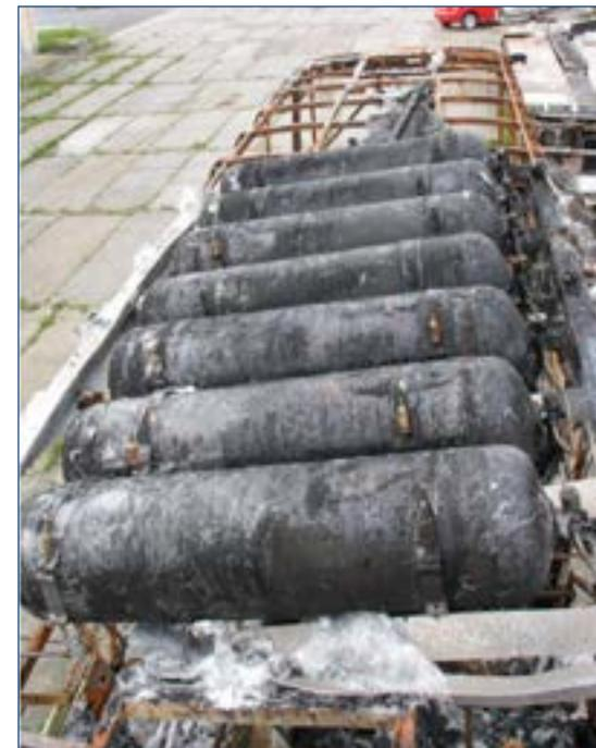
Figure 3 – CNG cylinders on the roof of the bus.
