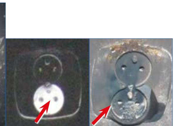
Figure 5 - Detail of socket immediately after the fire and during examination by fire investigator.
