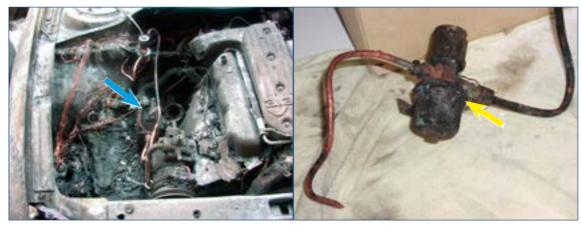
Figure 2 – Car engine - solenoid valve (blue arrow). Figure 3 – Place of the gas leak - fitting of the solenoid valve.
