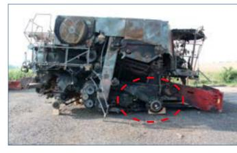
Figure 1 – Case 9230 harvester with marked criminalistics focus.
