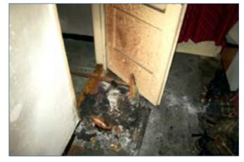
Figure 2 - Point of origin - burned vacuum cleaner in front of the toilet door.
