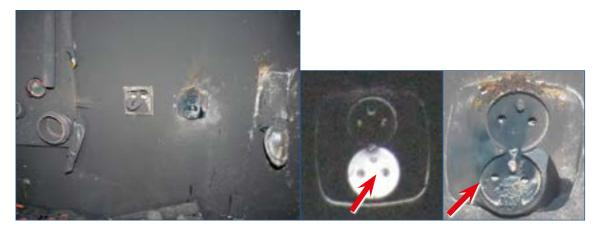
Figure 4 - Socket during examining by fire investigator.
