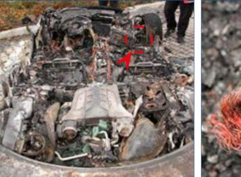
Figure 3 - Interior view on the Audi R8 Torus with marked outbreak where the power cable insulation has been damaged.
