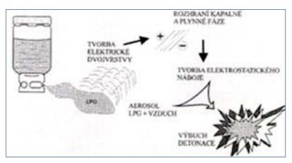
Figure 5 - Specific LPG risks are listed on the diagram.
