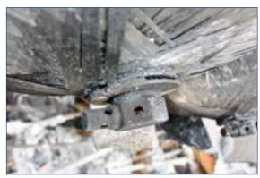
Figure 4 – Thermal fuse.
