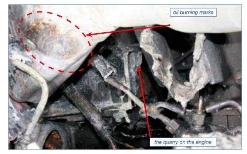
Figure 3 - View of the engine block and exhaust gas collector.
