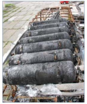
Figure 3 – CNG cylinders on the roof of the bus.
