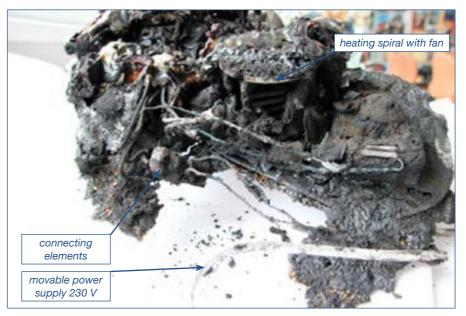
Figure 3 - The point of origin on the base unit of the fruit dryer.
