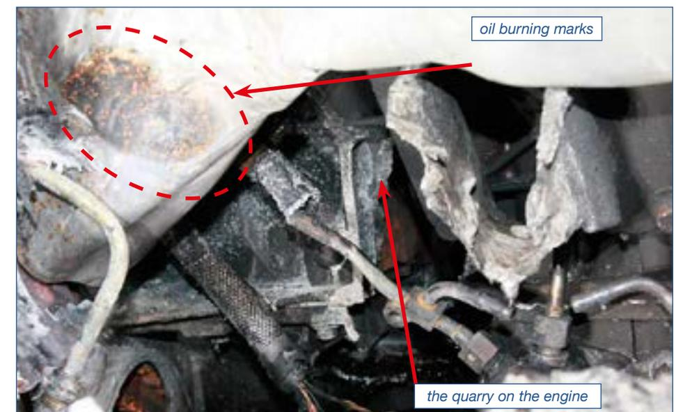
Figure 3 - View of the engine block and exhaust gas collector.
