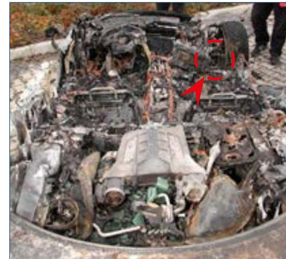
Figure 3 - Interior view on the Audi R8 Torus with marked outbreak where the power cable insulation has been damaged.
