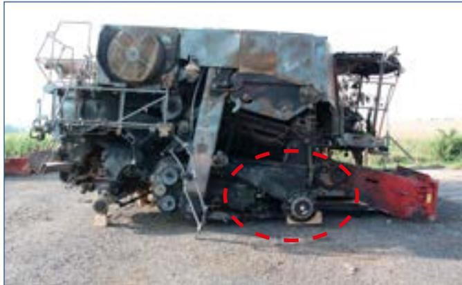
Figure 1 – Case 9230 harvester with marked criminalistics focus.
