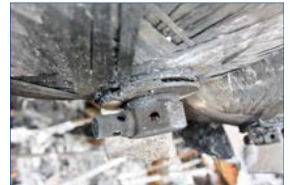
Figure 4 – Thermal fuse.
