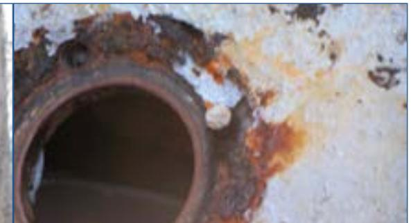
Figure 4 – Detail view on a screw which was grinded by angle grinder.
