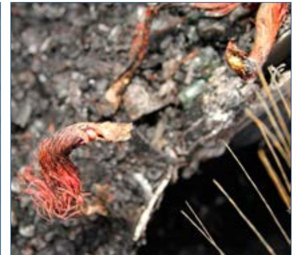
Figure 4 - View of the pearls in the form of Copper nozzles and thermal break of the cable core.
