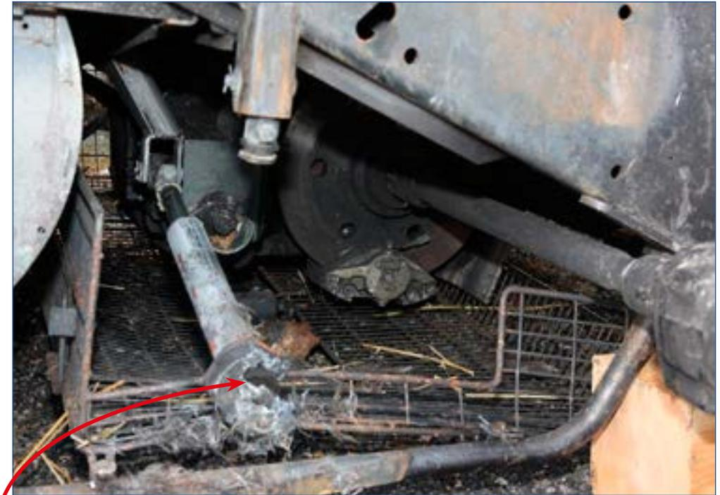
Figure 3, 4 – Comparison of damaged and undamaged electromechanical system of harvesters sieve box.
