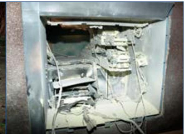
Figure 4 - View of the internal damaged part of the ATM.
