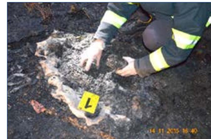
Figure 5 - Remnants of the fireplace under the vehicle, covered by vehicle insulation.
