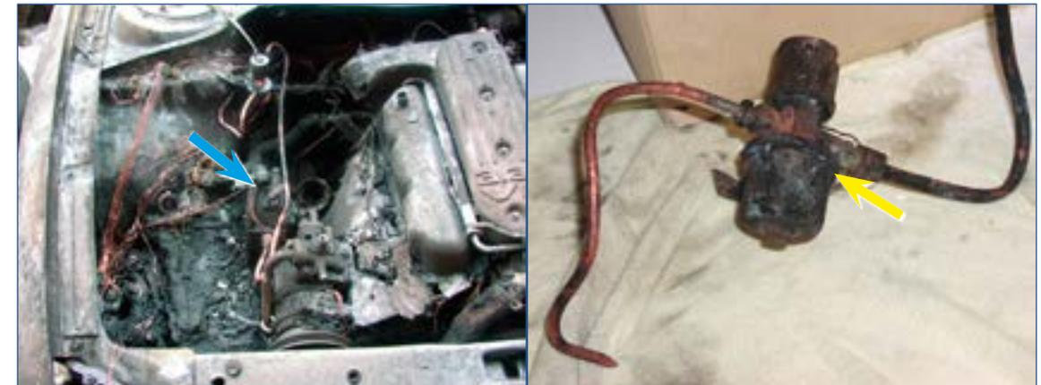
Figure 2 – Car engine - solenoid valve (blue arrow).
